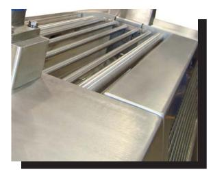
Heavy Steel Plate / Continuous Sanitary Welds
