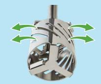
The high velocity radially discharged streams impact the slower moving tank flow for additional hydrodynamic shear and circulation, thus ensuring high flow, with no dead spots in the mix tank.
